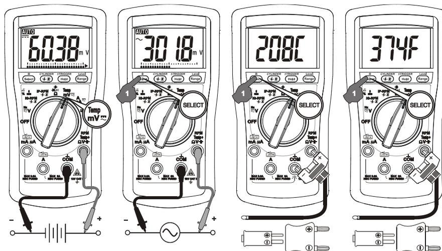
**Note:** Be sure to insert the banana plug K-type temperature bead probe Bkp60 with correct  $\pm$  polarities. You can also use a plug adapter Bkb32 (Optional purchase) with banana pins to K-type socket to adapt other standard K type mini plug temperature probes.
