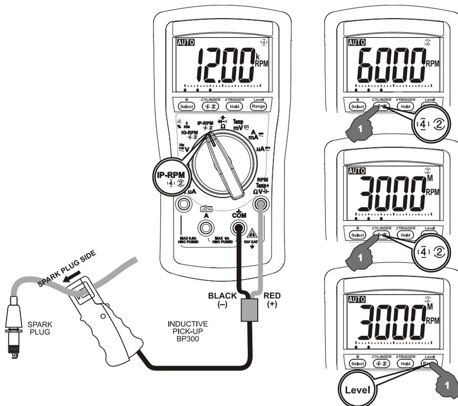
Press  $\bar{4}$   $\bar{2}$  button momentarily to select through **RPM  $\bar{4}$**  for 4-stroke, **RPM  $\bar{2}$**  for 2-stroke and DIS, and **RPM  $\bar{2}$  M** for special 2-stroke waste ignition engine
