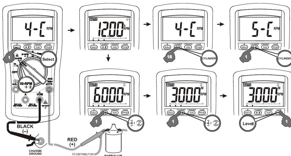
Press  $\text{4}$   $\text{2}$  button momentarily to select through **RPM<sup>4</sup>** for 4-stroke, **RPM<sup>2</sup>** for 2-stroke and **DIS**, and **RPM<sup>2M</sup>** for special 2-stroke waste ignition engine
