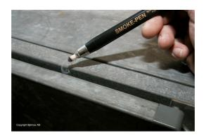
The Smoke Pen works like a mechanical pencil. A patented smoke-emitting wick is inserted into the convenient to use pen, adjust the wick to provide 10 mm or 3/8" of exposed wick, light the wick with a match or lighter.
